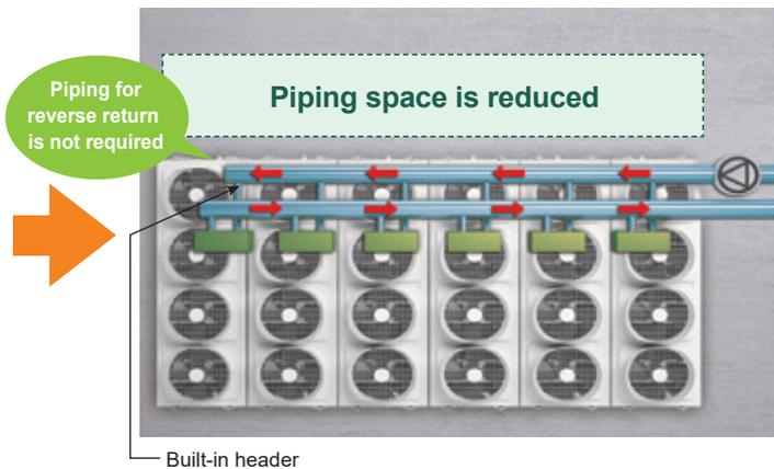
The size of the piping for the built-in header type is large to reduce pressure loss in the piping. It is unnecessary to prepare the piping for reverse return. This helps to reduce piping space and equipment cost.
