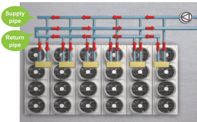
With standard piping construction, the customer must determine and design the return piping. The supply pipe and return pipe of each unit should have the same overall length and piping resistance to keep a balance among the flow rates to the units. Therefore, piping space and equipment costs are required.
