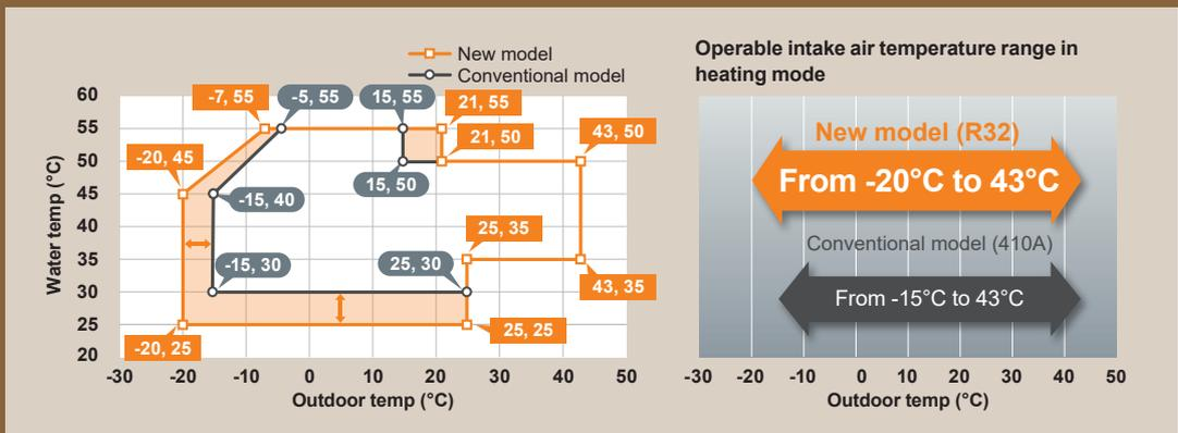
\*The function to protect the units is triggered when the units are operated at a temperature outside the operating temperature range listed above. When this happens, the units will either be operated in the capacity-save mode or come to a stop and will be unable to supply water at the target temperature. Also, the units may be operated in the capacity-save mode at the start of heating operation (while warming up) due to the protection function.
