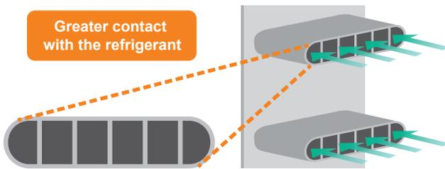
The fins inside the flat tube divide the flow of refrigerant into multiple paths and improve heat-exchanger effectiveness. Flat tubes reduce wind resistance and increase the number of piping stages, resulting in an overall improvement in heat exchange efficiency.
