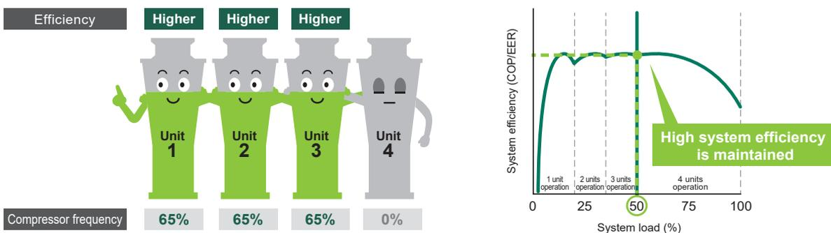
Each unit has inverter compressors, and the operating frequency and the number of units to be operated are controlled to maximize the operational efficiency of each unit based on the total system compressor frequency for the entire group. This function improves system efficiency when operating at low to medium loads.
