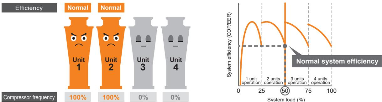
Without optimum frequency control, it is only possible to turn the unit on or off, and compressor frequency cannot be adjusted according to the required capacity.
