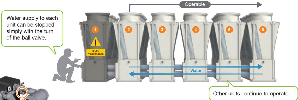
**Water heat exchanger (built-in header types only)**
