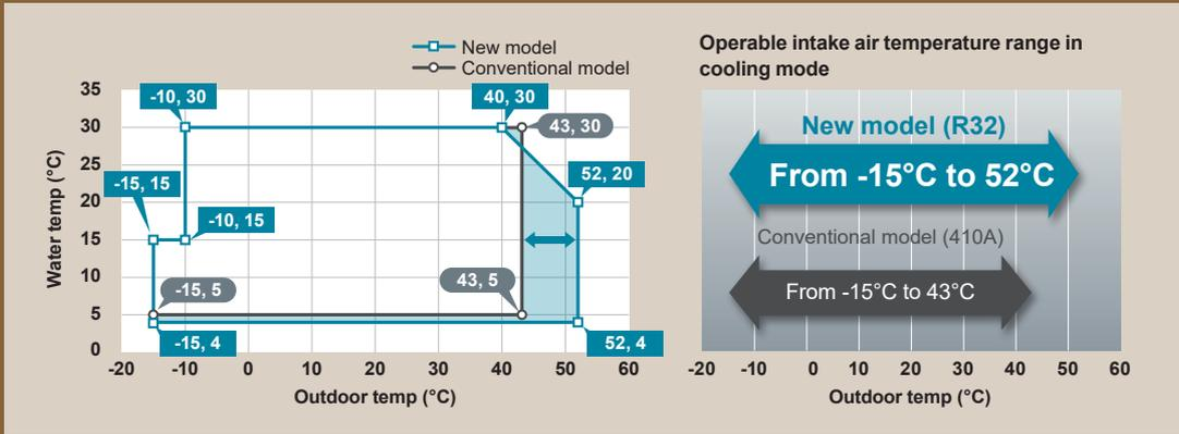
In built-up areas with a high density of buildings, wind may be blocked, causing an accumulation of warm air in the vicinity of the unit. The new model is guaranteed up to 52°C, so operation remains stable even in such situations.
