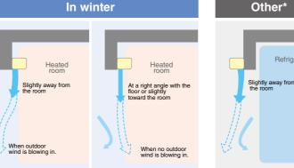
\*The inside temperature differs significantly from the outside temperature (such as in the case of a refrigerator.) (Make sure there is nothing in the way of the generated wind.)
