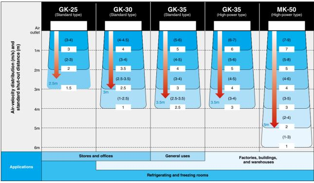
\*The figure in  $\square$  indicates average velocity (m/s) at the given distance
