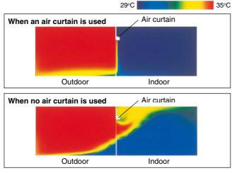
Experiments have proven that the air curtain effectively blocks 70-90% of outdoor heat or cold air, where a glass panel is assumed to block them 100%. (The effect may vary according to the difference between indoor and outdoor temperatures, whether there is wind outdoors, or the height of the air curtain.)
