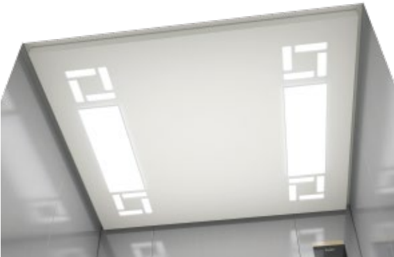
CD0 LED Lighting: Milky white thin lamp cover + milky white lighting panel Material: Sheet steel with painted finish (C033) + milky white resin panel Note: For bed elevators, this ceiling model refers to as BD0
