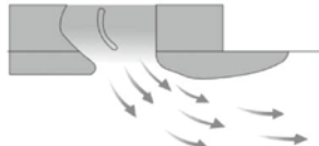
Optimized air diffusion type by Climaveneta The upward airflow is limited
