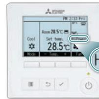
"HiPower" is displayed on the monitor during high power fan speed mode.
