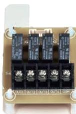
RVX3's PCB has only 1 output terminal. By using PZ-4GS-E, 4 more output terminals can be added to RVX3.
