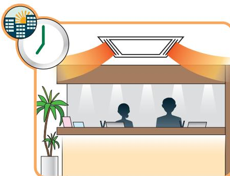
When the temperature sensor detects a certain amount of differential between the room temperature and the set temperature, the operation of all indoor units in the system is switched from heating to cooling.
