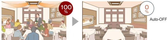
\*No occupancy Auto-OFF mode is not available when multiple indoor units are operated by one MA remote controller.
